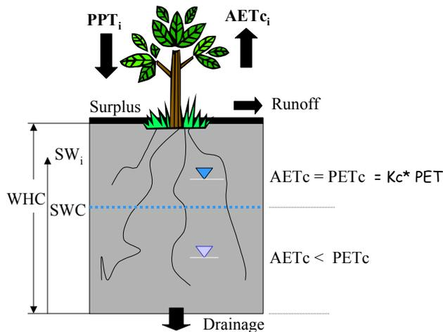
Figure 1: Components of a Crop Water Balance Model
